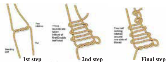
Figure 1: Meltzer knot, 2:3:2 (Two hitches, Three winds, Two half locking hitches)
